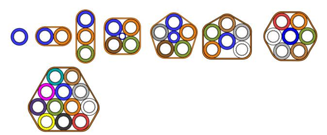
**GENERIC PRODUCT DESCRIPTION**: Assemblies of strong 12/8 polyethylene (PE) microducts (m/d), each with low friction performance. These m/ds will accept all blown fibre products that can be installed into the more traditional 10/8 m/ds. The 4-way has a 5/3.5 m/d in the centre. The 5-way has a strong 8/3.5 m/d in the centre.
