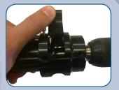
Attach prep/strip tool to drill. Open blade lever and lock with pin. Insert cable and actuate drill.
