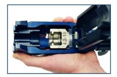
Press the plastic removal tool behind the adapter. Squeeze the release lever and remove the adapter.
