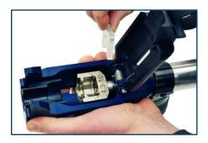
Squeeze the lever arm until there is enough space to insert the plastic removal tool.
