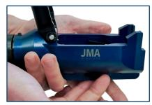
Slide the bottom cable insert backward until it can be removed. Repeat this step with the top cable insert inside the hatch.
