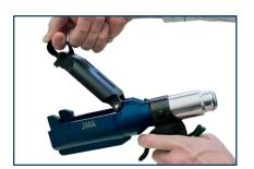
Open the top hatch by pulling upward on the release strap.
