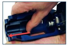
Install the bottom cable insert into the front of the frame as shown. Repeat this step with the top cable insert inside the hatch.
