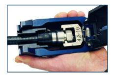
Insert the cable and connector into the frame and close the top hatch. Follow the supplied connector installation instructions.
