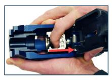
Place the interface insert into the rear of the frame. Press firmly toward the back of the unit.
