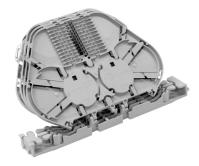
FIST<sup>™</sup> Splice Sub-assembly kit with 4 slim element trays, each for holding up to 9 primary coated fibers, with Heat Shrink type splice holder and universal 1x8 splitter holder
