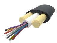
LightScope ZWP® Self-Supporting All-Dielectric Outdoor Drop Cable, 1–12 fiber Arid Core construction, central loose tube, no ripcords
