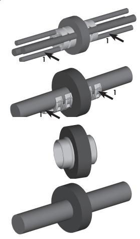
1.2.5 Wrap the length of gel tape around the centre of the branching plug or port reducer. Do not stretch the gel sealing tape during wrapping.
