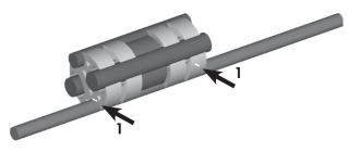
1.1.4 Install the branching plug onto the cable(s) in the appropriate port having removed the blanking rod(s) (see selection table on page 1).Note: taping the cables together each side of the plug will help to keep the plug in position (1).
