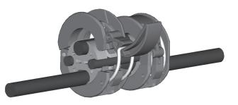
1.2.1 Install the 2 hinged clamps over each of the rubber sections of the branching plug; the raised ridge on the inside of the clamps fits into the groove in the rubber of the branching plug or into the groove in the plastic of the port reducer.
