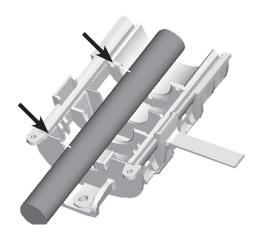
1.1.2 For large and small closures centre the bottom half of the closure around the joint and mark the position of the inner and outside edges of the branching plug recess onto the cables.
