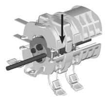
1.3.4 The closure lid has location pegs at each corner that locate into slots at each corner of the base- see above.
