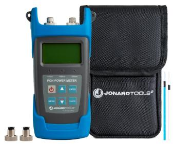
Designed to perform live testing with OLT equipment, this PON Power Meter with APC connectors is perfect for use during FTTx/PON service turn-up or maintenance. It is able to simultaneously test and measure the signal power of voice, data, and video connections, and is essential for the construction and maintenance of PON systems. Features the following:
