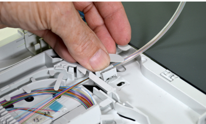
7.2.4. Mount the tube holder in the tray. A second tube holder can be mounted, if needed.
