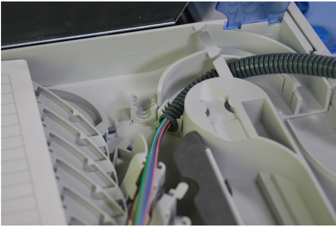
6.6. Guide the flex and the 900 \mu\text{m} fibers to the splice tray. Fix the flex tubes in the flex tube holder.
