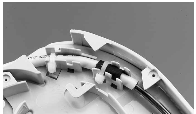
5.2.1 For ease of installation start with the bottom tray. If possible apply 1 wrap of foam tape around the IFC, just before the jacket end (This foam prevents from easy pull-out and provides protection to the fibers inside). Attach to the tray with 2 small tie-wraps. At least 1 tie-wrap should be on top of the foam tape. Cut the excess length of the tie-wrap. Make sure the tie wrap knob is at the side of the IFC. Don't squeeze the fibers.
