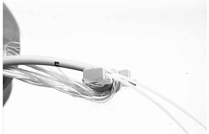
5.3.8 In case of pigtails with a limited amount of Kevlar (typical outside diameter < 2.4 mm): wrap the Kevlar twice around the inner part. Bring the Kevlar of 2 neighboring pigtails together and pass the Kevlar between both pigtails. Repeat for the 2 other pigtails. Always install 4 pigtails per GTU.
