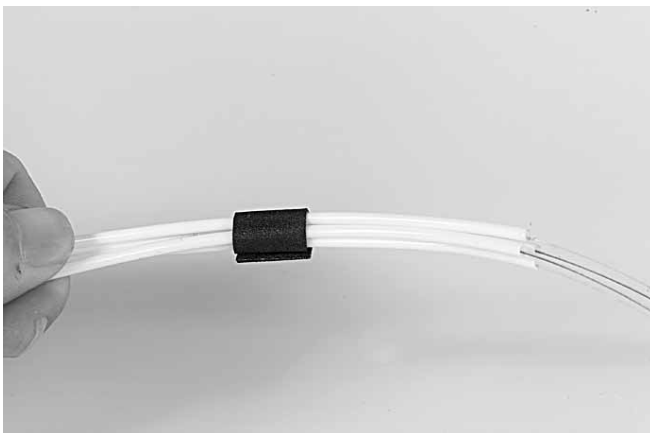
5.1.12 Strip the loose tubes and place 1 layer of foam around all the tubes at 50 mm from the end of the tubes.
