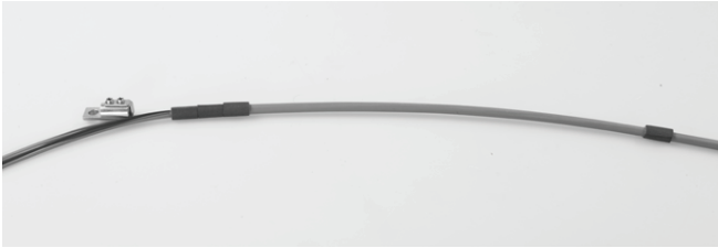
5.1.11 Also apply foam tape around the cable approximately 38cm from the point where cable is stripped.
