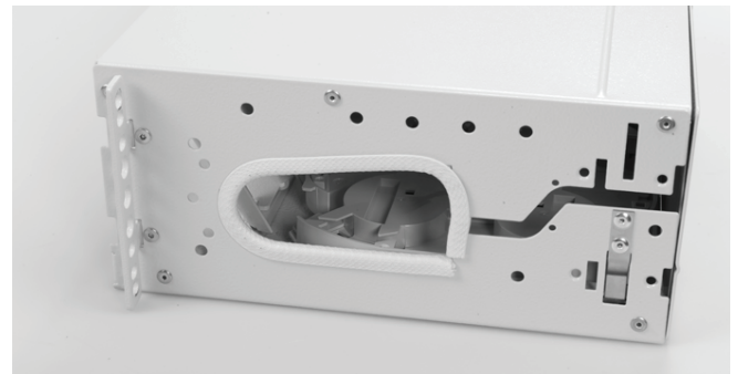
4.8 Install the edge protector on the entrance cable area side.
