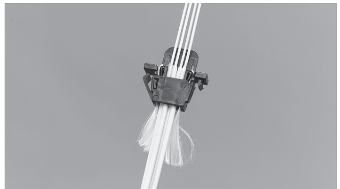
5.15 Cut the excess of the Kevlar, leaving 5-10 mm.
