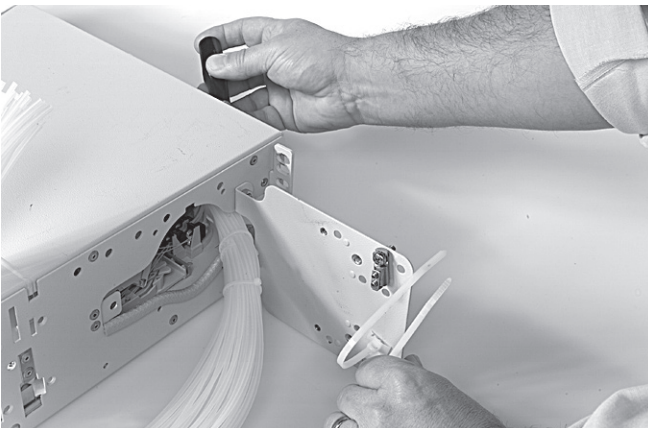
4.2.14 Install the side termination bracket on the shelf, before mounting the shelf in the rack.
