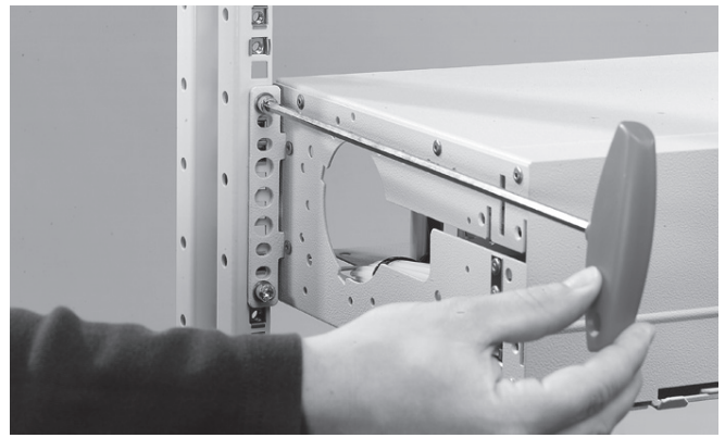
3.1.4 Mount the shelf using the FACCC-ALLEN-KEY.
