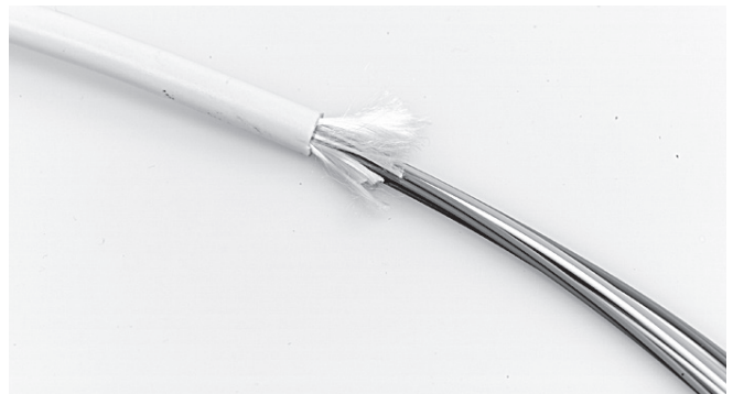
4.1.34 Remove the cable jacket over approximately 1.7 m.
