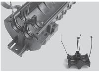
5 Insert the tie wraps in the cavities of the bottom part (2 at each end) and the 4-out cable separator. Note: The tie wraps will keep the cables and plugs in place during installation.
