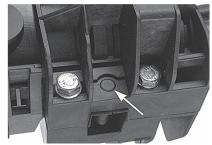
21 The indicator should protrude the top half shell and be at the level of the top part as shown in picture.
