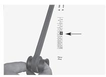
16 For unused cable ports, plugs need to be installed. Wrap gel tape around the centre of the plugs. The required length is marked on the measuring tape (black square) as shown.
