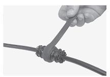
15 Wrap the gel tape around the cable in between the 2 axial pull strips. Note: Do not stretch the gel tape during wrapping. Repeat steps 8 to 15 for all cables. **Note:** For ease of installation, long gel tapes
