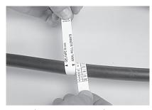
8 Use the measuring tape to determine the required length of the axial pull tape. The measuring tape indicates the number of axial pull elements needed.
