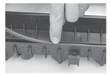
3 Insert the longitudinal O-ring seals in the grooves of the bottom half shell.
