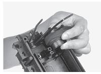
17 Insert the plugs (with gel) in the bottom shell and tighten the tie wraps. Make sure the knob of the tie wrap is on top and cut away the tail.
