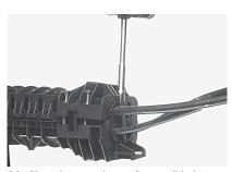
20 Close the central part. Screw all bolts tight, starting with the two mid bolts at both ends. Do not screw each bolt tight completely one after the other. Screw all bolts tight sequentially.
