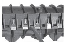
22 Make sure there is no gap between the half shells at the position of the bolts and all snapfits are locked.
