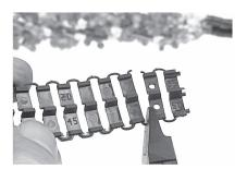
9 Cut the axial pull tape to the measured length.
