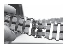
10 In case the measured length exceeds the max. length of one tape, two or more axial pull tapes can be connected together.
