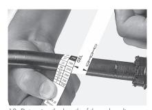
13 Determine the length of the gel sealing tape using the measuring tape (mm).
