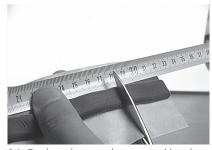
14 Cut the gel tape to the measured length.
