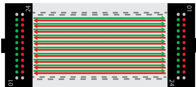
Figure 4: 100GBASE-SR10 full duplex operation on 20 fibers
