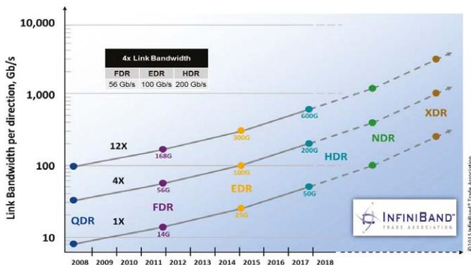
SDR—Single data rate      FDR—Fourteen data rate      HDR—High data rate
