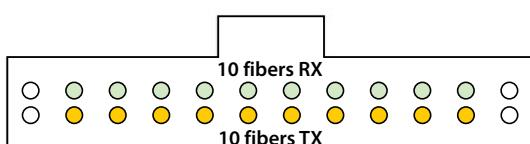
Figure 5: MPO connector pinout for 100GBASE-SR10
