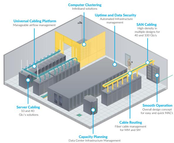
Figure 8: Cabling system infrastructure
