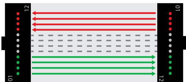
Figure 2: 40GBASE-SR4 (40GBE) and 100GBASE-SR4 (100GBE) full duplex operation on eight fibers
