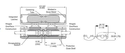
For direct buried or aerial\* splicing of Series 7 and 11 coaxial cables, long body F-81 and sealed connectors.
