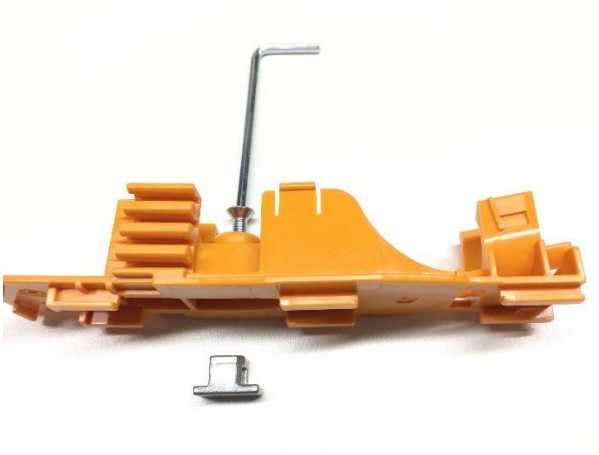
10.5.1 Install screw and strength member connector.
