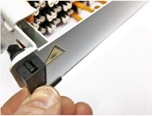
10.1.5 For locking the cover, push the latch down.
