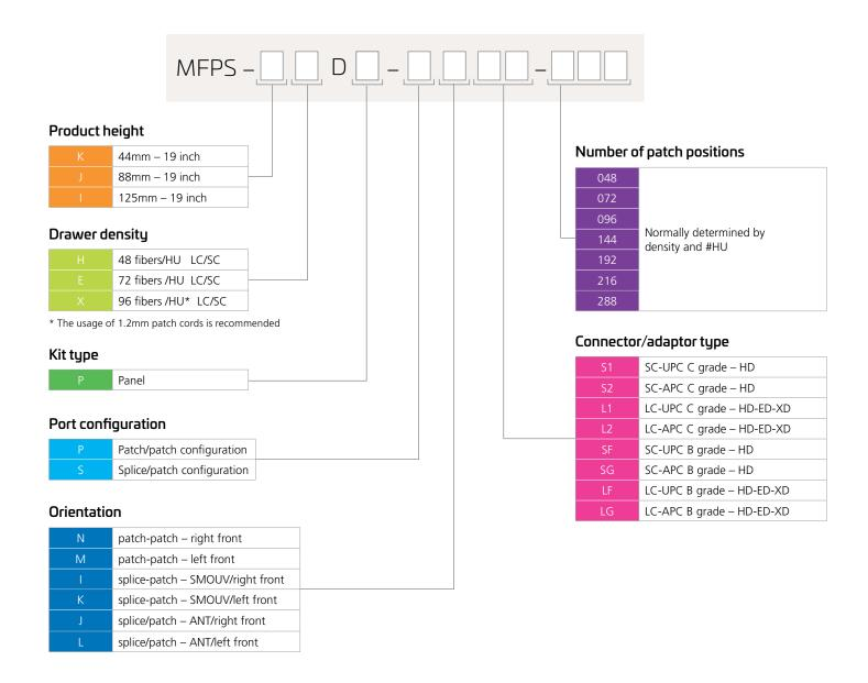
The MFPS family of solutions provides a range of configurations, densities and sizes. So you have one reliable solution for all your FTTx patching applications.
