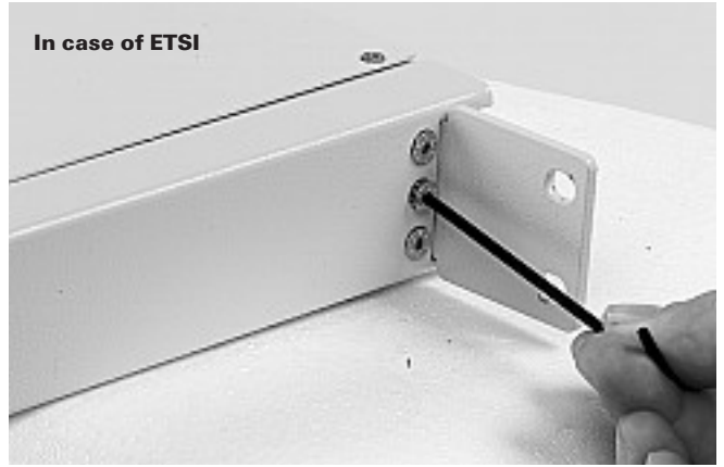
3.1.3 Install the mounting brackets on the correct position. Respect correct orientation.
