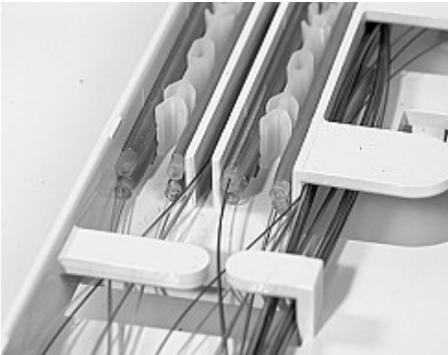
3.7.3 Rotate the FOSC-tray \pm 45^\circ .
