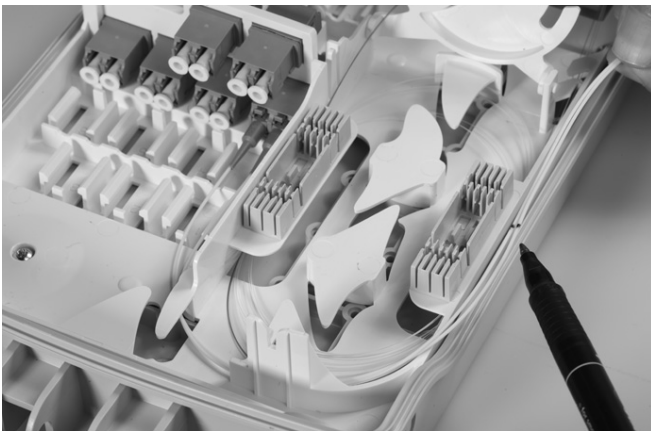
2.3.4 The pigtails should be stripped when entering the storage area in a straight line.
