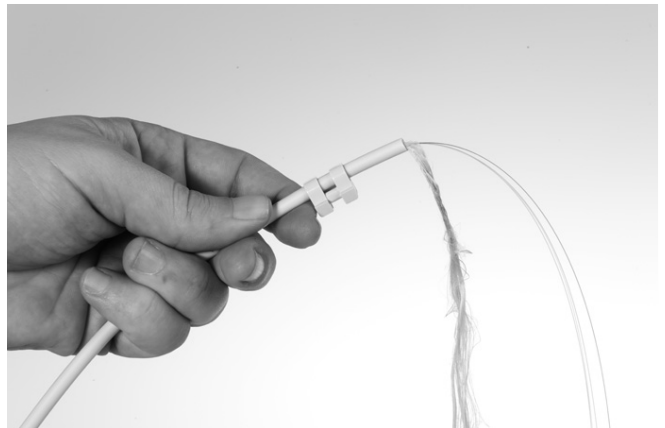
2.1.2 Install the termination unit onto the cable.
