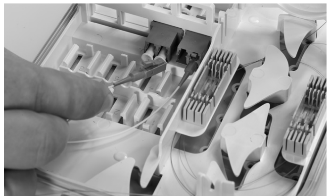
2.3.3 Connect the pigtails into the designated adaptors.
