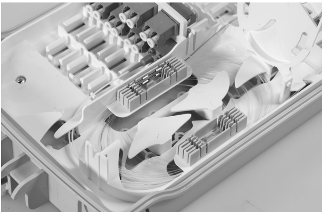
2.3.5 Splice the pigtails and store the splices in the splice holder, first use the left holder as shown on the picture, this to avoid crossings when adding a new incoming cable.
