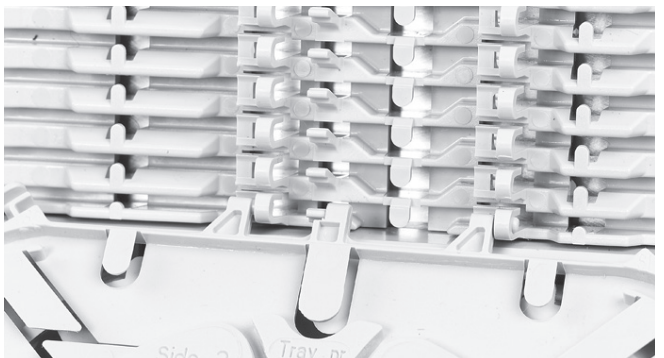
4.4 Place a tray in the wraparound groove plate; do this by pushing the lip on the groove plate (lowest possible position) slightly down with the tray and move the tray lateral into the hinge-cavities of the groove plate. To snap the High Capacity Single Element tray (HCSE) in the W/a single fiber groove plate leave always one hinge facility open between Fasblock or previous tray and the HCSE-tray.
