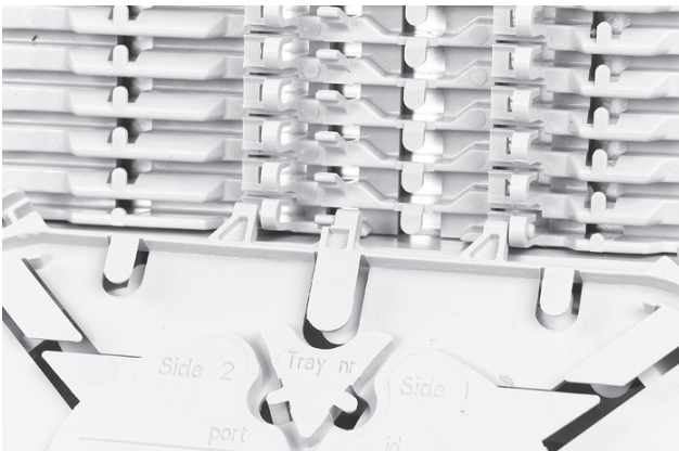
4.3 Place a tray in the wraparound groove plate; do this by pushing the lip on the groove plate (lowest possible position) slightly down with the tray and move the tray lateral into the hinge-cavities of the groove plate. To snap the High Capacity Single Element tray (HCSE) in the W/single fiber groove plate leave always one hinge facility open between Fasblock or previous tray and the HCSE-tray.
