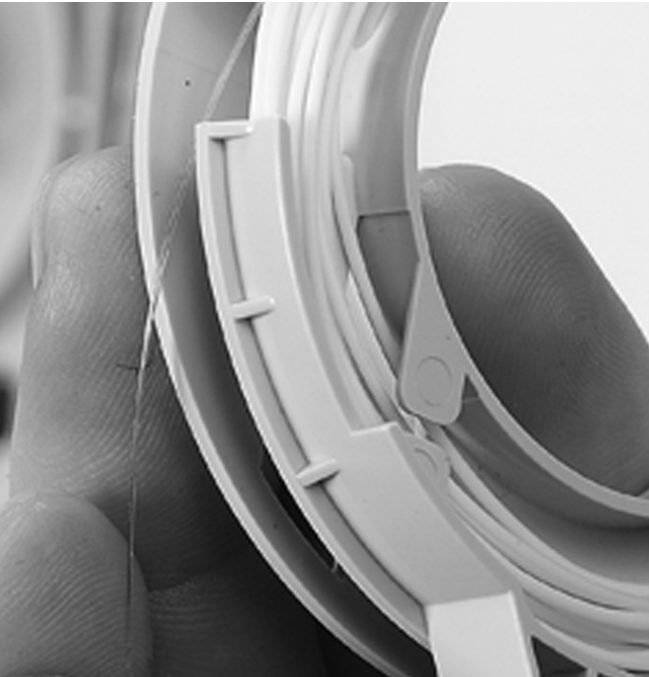
1.2.10 Route the feeder cable fiber to the backside of the tray as shown in the pictures.
