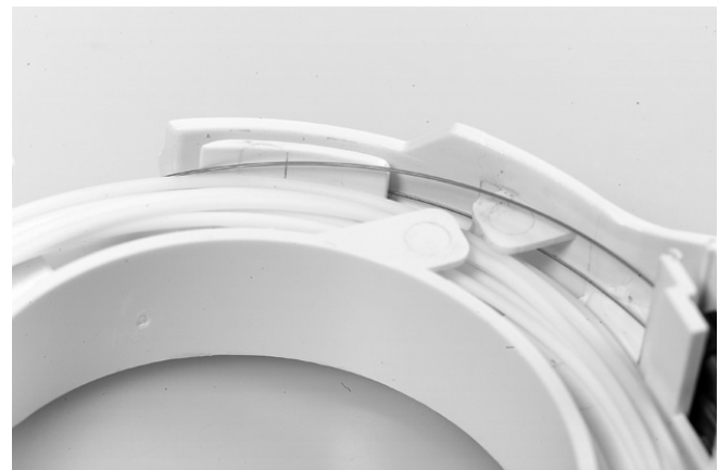
1.2.11 In case of LC duplex, route the feeder cable fiber of the second splice to the backside of the tray as shown ( not underneath the lip and not in the groove).
