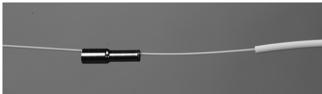
4.1 Slide a metal boot over the transportation tubes on both sides of the fiber.
