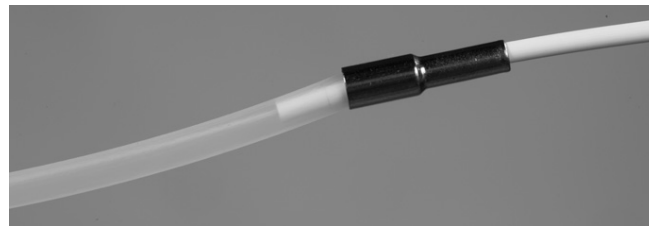
4.4 Slide the transportation tube over the fiber. Secure on both sides with the metal boots.
