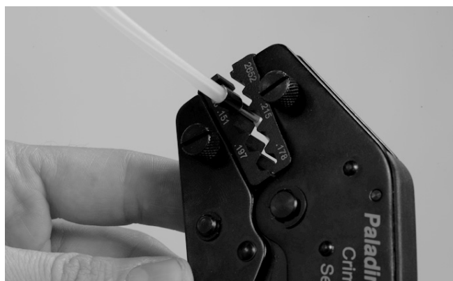
4.4 Slide the transportation tube over the fiber. Secure on both sides with the metal boots.
