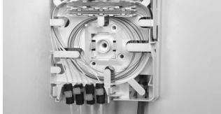
6.6 No connectors, store the overlenght of the pigtails and fiber cable in the storage area.
