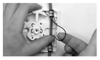
4.2 Pull out the required fibers by using the thumb to control the bending and one finger for pulling .
