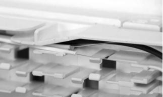
6.2 Recommended to strip the 900 micron to 250 micron half way the splice holder, in case of semi-tight pigtails. In case the pigtail is tight, only 0.8 m can be stored in the storage area.
