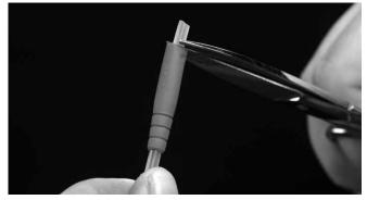
5.3.3 Push the transportation tube trough the boot and cut away at the edge of the boot.
