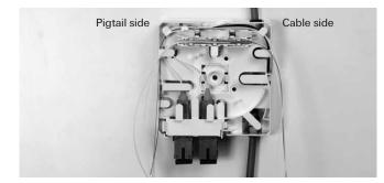
6.5 Install the splice protectors into the splice holder. Check the orientation of cable-pigtail side to avoid crossings.
