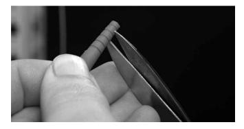
5.3.2 Cut away some part of the boot if needed for pushing through the transportation tube. Cut maximum 2 elements of the boot.
