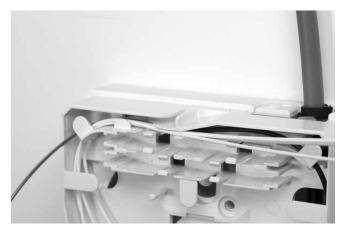
6.1 Route the 900 micron pigtail behind the splice holder.
