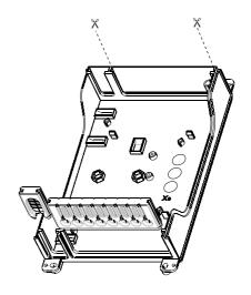
3.1 Break out the ports needed, For breaking out the ports, first cut with the scissor.
