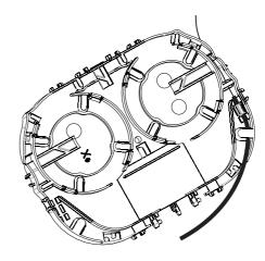
4.7 Separate the fibers from the ones to be stored and route these fibers to the top side of the tray.
