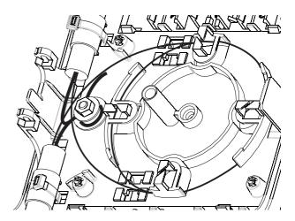
4.3 Cut the Kevlar over a length of 150 mm and terminate the Kevlar
