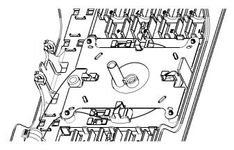
4.5 For the uncut fibers in the butt application storage can be done in the bottom of the box (max. 700 mm). Install the cover to protect these fibers.
