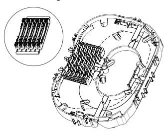
6.1 Install the splice in the splice holder and then store the overlength in the tray. Different splice protectors can be used.
