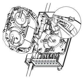
4.6 Install the transportation tube over the fibers. Slide the snap fit over the transportation tube. Lock the transportation tube into the securing position. Store the incoming fibers in the bottom side of the tray.
