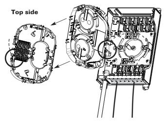
$5.3\,$  Cut the appropriate seal by using a scissor. First install the bracket starting from 1 to 4 following with 5 to 8. Route the 250/900 micron to the top side of the tray.
