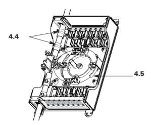
4.4 Wrap 1 layer of foam on the securing positions of the cable. Secure the cable with tie-wrap on this positions onto the box. Install the cable seals onto the cable.
