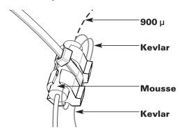
5.2 Wrap one layer of foam (20 mm) on the securing position if needed. Terminate the Kevlar by securing the cable/pigtail onto the bracket with tie-wrap. Depending the amount of Kevlar, it needs to be wrapped twice around the bracket.
