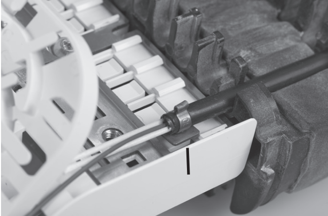
5.1 Remove the jacket at the indicated point and take out the needed fiber, store the rest in the dedicated zone.
