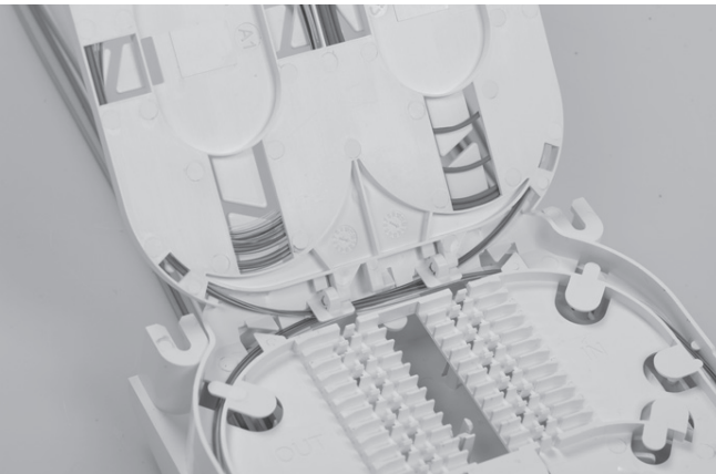
4.1.9 Install the first splice tray and lift the top part, route the fiber bundles via the groove plate in the bottom (splice) part of the cassette. use the outer (left en right) "channels "to go to the top part for storing the unused fibers.
