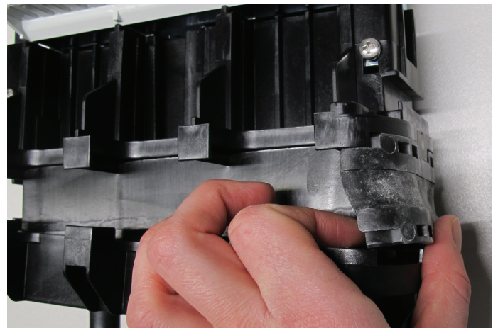
9.3.4.3. Insert the wrapped metal band in the CTU slot.
