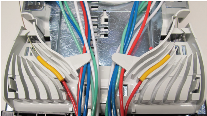
11.3.8 Press the piece of orange tubing in the groove on top of the tube/subunit.
