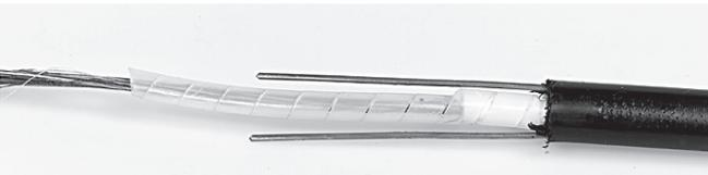
4.2.39 Put the spiral tube on the cable
