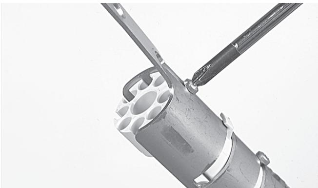
4.2.32 Loosen a little bit the screws such that one can position the strength members stop according to the position of the strength members and remove the break-out part.
