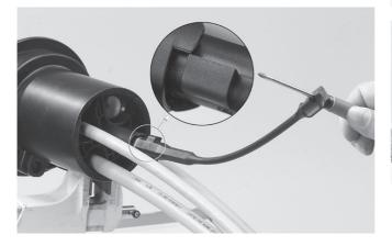
5.7 Turn the "tail" clock-wise until it dead ends at the positive stop. A screwdriver can be installed through the hole in the "tail" to tighten the seal.
