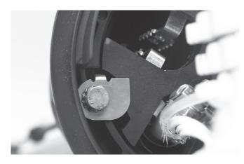
5.5 Secure the frame to the base with the two metal latches.
