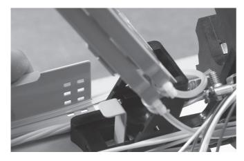
4.4.15 Secure one end of the tube to the tray and route the transportation tube to the basket. **Note**: make sure the tube makes a smooth bend around the tray tower.
