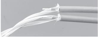
4.1.1 Make a window cut of 2.2 m. Cut the strength member at a distance of 40 mm from the jacket.
