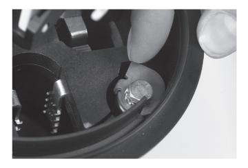
$3.2 \ {\rm Loosen}$  and turn the two metal latches that secure the frame. Take out the frame.
