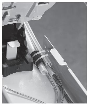
$4.4.1\,1\,$  Route the fibers to the appropriate trays through transportation tubes.
