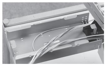
4.4.16 Secure the transportation tube and loose tubes to the basket with tie-wraps.
