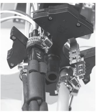
4.3.7  $\,$  Position the teeth of the cable retention brackets onto the grommet.
