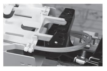
4.4.7 Secure the transportation tube to the tray with tie-wraps. Note: if necessary mark and remove the tube excess. The tube is 15 mm onto the tray and has to make a smooth bend around the tray tower.
