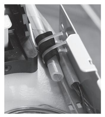
4.4.10 Secure the tube/spiral to the basket with tie-wraps. **Note**: when spiral is used, put some foam on the spiral underneath the tie-wraps.
