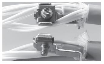
4.3.1 Secure the strength member into the strength member attachment.
