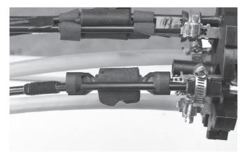
4.3.10 Insert the drop cable assembly through the FOSC 450 closure base and position it into the designated port.
