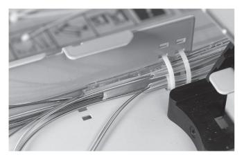
$4.4.18\,$  Secure the central core (150 mm long) to the basket with tiewraps.
