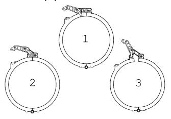
3.1 Remove the dome to base clamp. Remove the dome and O-ring.
