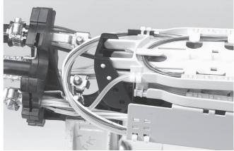
4.4.17 In case the loose buffer tubes are not kink sensitive, they can be routed onto the tray following the above shown path. Wrap tape around the tube(s) before securing to the tray.
