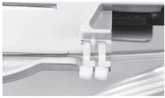
4.4.2 Slide the appropriate transportation tube over the loose tube and route to the tray. Mark at 15 mm from the tray edge. Remove the tube excess from the mark and secure to the tray with tie-wraps.
