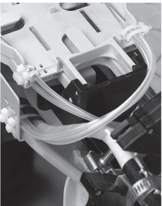
4.4.12 Secure the transportation tubes to the tray with tie-wraps. **Note**: if necessary mark and remove the tube excess. The tube is 15 mm onto the tray and has to make a smooth bend around the tray tower.
