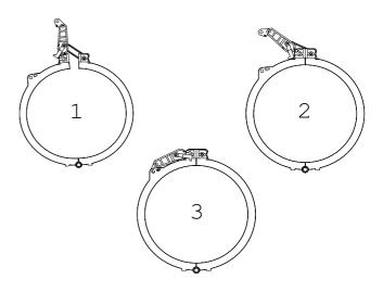
9.3 Install clamp around dome/base interface. Use the feet of the clamp handle to close the gap in the clamp.
