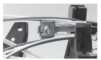
4.3.5 Secure the strength member(s) into the strength member attachment.
