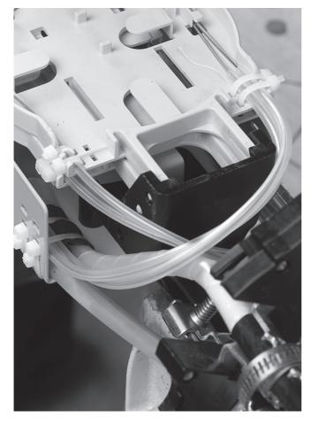
4.4.19 Route the fibers through the transportation tubes to the appropriate tray(s). **Note**: make sure the tubes make smooth bends around the tray tower.
