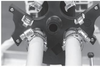
4.3.4 Place the cable(s) between the cable retention brackets. Secure the cable(s) with the supplied hose clamp(s)
