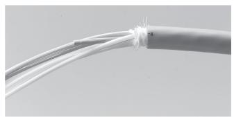
4.2.1  $\,$  Remove the jacket over a length of 1.2 m , cut the strength member at a distance of 40 mm from the jacket.
