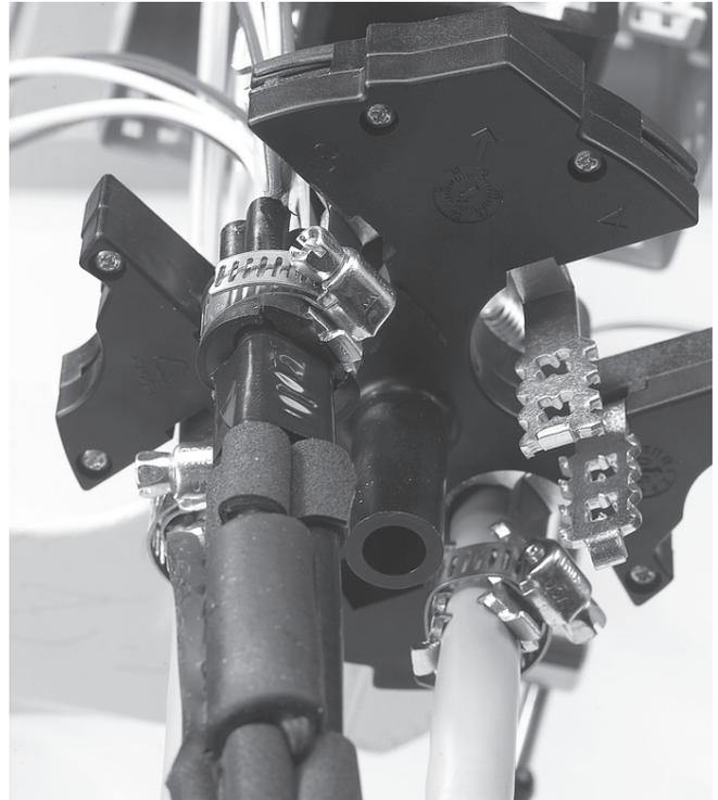
4.3.7 Position the teeth of the cable retention brackets onto the grommet.
