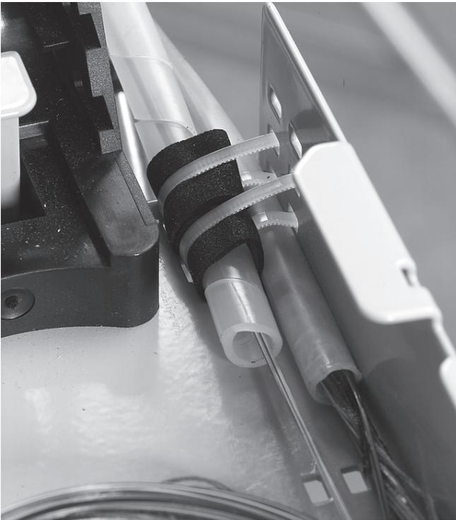
4.4.10 Secure the tube/spiral to the basket with tie-wraps.
