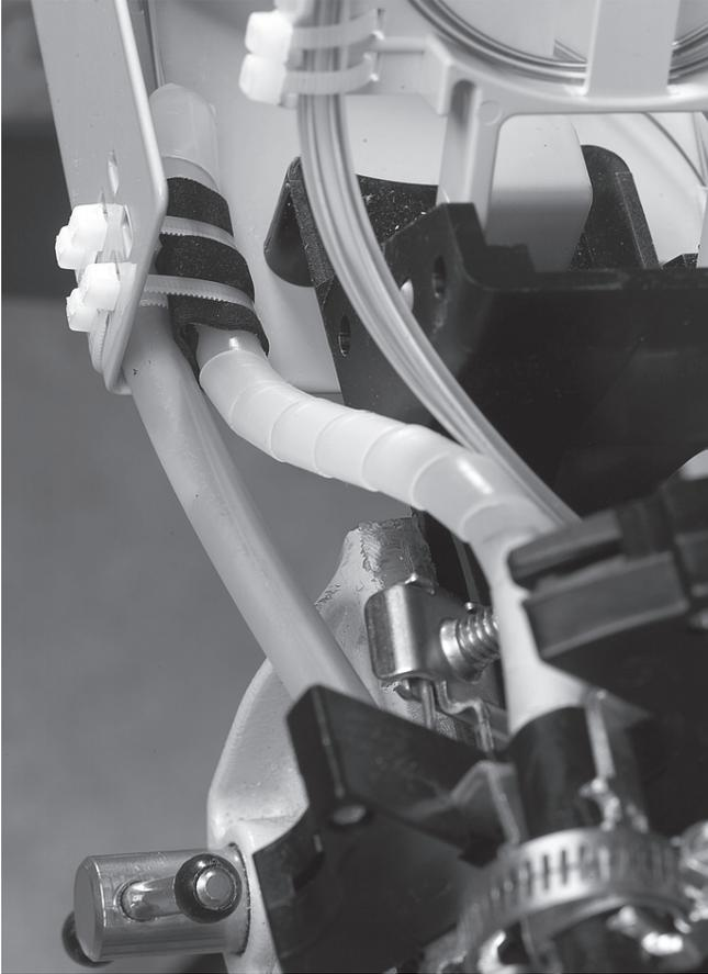
4.4.9 Slide the appropriate transportation tube/spiral tube over the central core (uni-tube) and route it to the basket.
