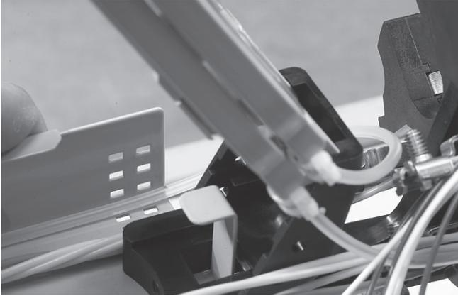
4.4.15 Secure one end of the tube to the tray and route the transportation tube to the basket.
