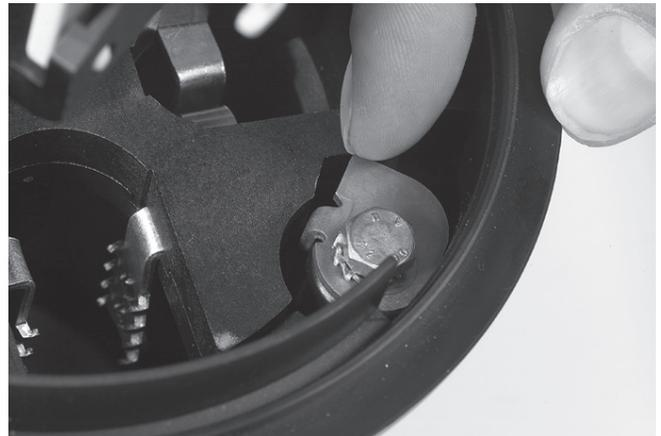
3.2 Loosen and turn the two metal latches that secure the frame. Take out the frame.
